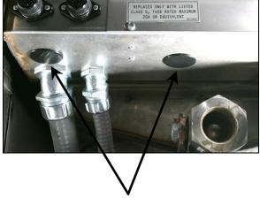
Bottom of Component Box Drain Valve Plugs Installed in Component Box
